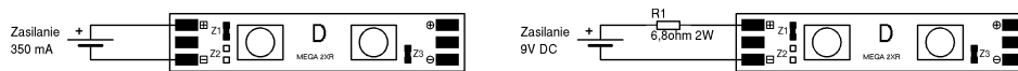
Fig. 4. Single module connected to current power supply (350/700mA) or voltage power supply (9V DC).
