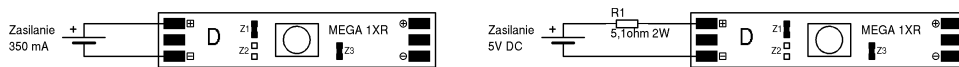
Fig. 4. Single module connected to current power supply (350/700mA) or voltage power supply (5V DC).
